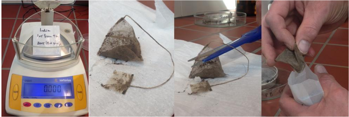
Figure 5: Work steps 4.1 – 4.6 – Reprocessing of the collected tea.
