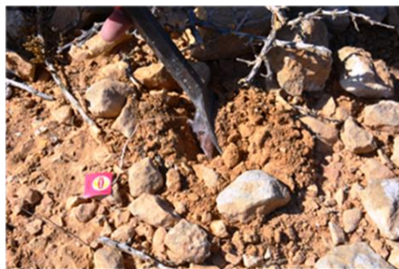
Figure 3b: Work steps 2.7. - 2.9 – Positioning of tea bags in the soil. Soil layers: a) organic layer (L =leaf litter layer, F =fermentation layer-where organic matter starts to decompose, H = humus); b) mineral layer (A = topsoil- mixture of organic matter and mineral matter, B =subsoil; c) parent material
